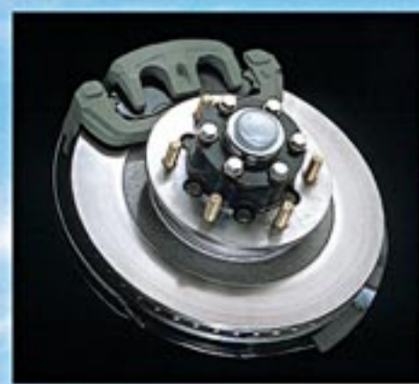
4-Wheel Disc Brakes: 2-Pot Ventiladed in Front, Solid Drum-in Disc Rear Brakes
