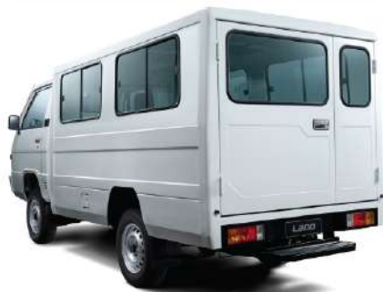
L300 Cab and Chassis shown with optional FB rear body and dual air conditioning system.
